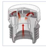
When using plumbing system underpressure can occur, that's when the HypAirBalance opens, allowing air to reach the system – thanks to which the pressure inside of the system balances itself.
