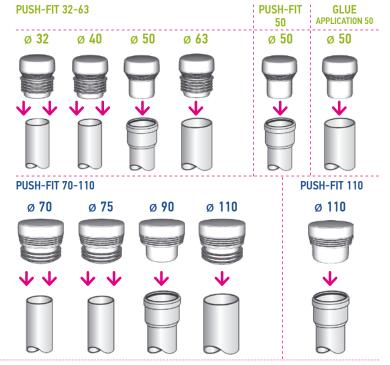
Properly installed HypAirBalance valve facilitates the free flow of waste water without draining the water from the siphon. It prevents unwanted infiltration of unpleasant smells from sewer lines into the room.
