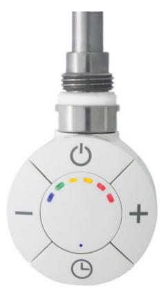
Electronic thermostat for electric towel heaters based on fluid heat transfer. The temperature is controlled by means of an external sensor. The **SMART** series has the heating element couples to the thermostat. The symmetry of the device enables both right and left side coupling to the towel heater. It is possible to choose between three predefined programs, as indicated in the guide for setting the operational times.
