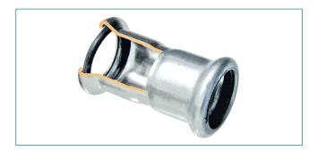
The connections at the pressfitting ends have a pocket in which the tube is inserted up to the stop end. A pressing machine with a suitably sized M jaw deforms, in a controlled way, the tip of the tube, assuring the unthreading rotation of the pipe under pressure.
