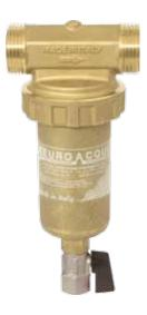
Mini Cleaning Filters - Sand collector cleaning filter with brass head, ring nut and vessel. Stainless steel cartridge. It cleans as it is equipped with a drain valve that removes the sand without having to take apart the filter.
